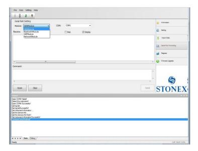
Fig. 5.25 - Serial Port Forwarding window
