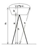
Fig. 4.5 - Different measures of the antenna height for S9 III PLUS
